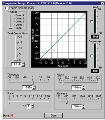
Figure 3.46. Compressor Setup window
